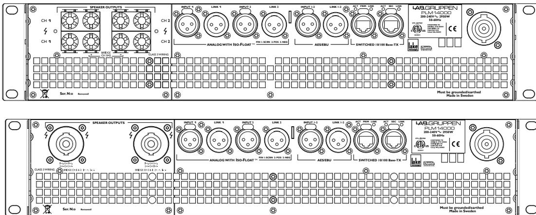
The PLM 14000 is available with either binding posts or an “embedded patch panel” with Neutrik speakON connectors (2 x NL4). Common connectors include; 2 x analog input XLR with switchable Iso-Float, 2 channels of AES/EBU with link-through capability for daisy chaining, 2 x EtherCON® for linking or redundancy. A 32 amp PowerCON® connector is used for mains supply.
