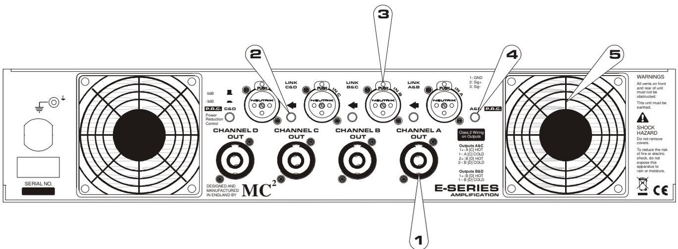
1: Channel A output Speakon socket: Normal output is on pins 1+ hot, 1- cold. Channel B's output is also wired to this socket to enable a single NL4 to provide both channels and to facilitate easier wiring in bridged mode. Channel B is wired pins 2+ hot, 2- cold.
